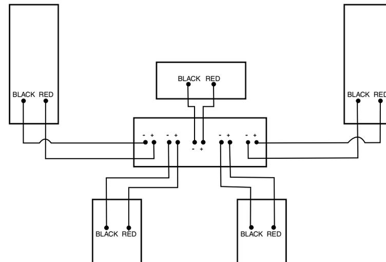
**FIGURE 4** Connecting Speakers to Amplifier or Receiver
