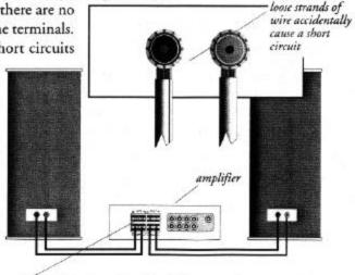
Your TF-400 Series Two's should be connected to your amplifier with the correct polarity. This insures that the pair will be in phase with each other, and will provide the best sound performance.
